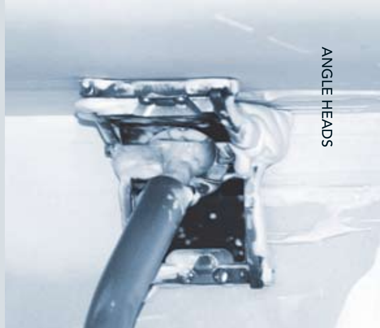
"Fail Safe" Locking Mechanism locks Angle Head on the ball
